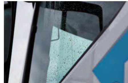
Water-Repellent Coated Pull Down Door Glasses
