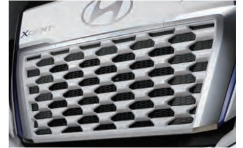
Mesh Type Radiator Grille with V-Shaped Matte Chrome Garnish
