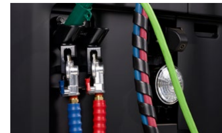
TRAILER CONNECTOR Placed at the rear for easy connection to the trailer. (North American SAE standard)
