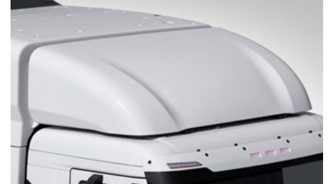
ROOF FAIRING / SPOILER Curvy roof fairing reduces drag and improves mileage.
