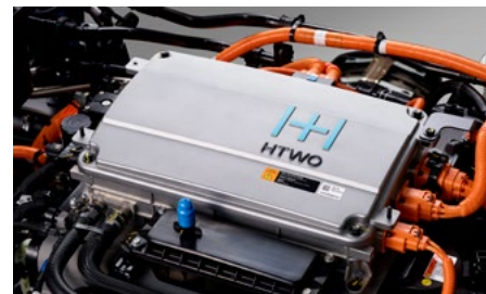
STACK 2 180 kW (2 x 90 kW each)
