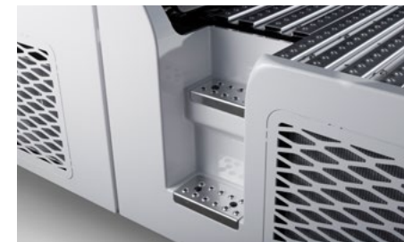
SIDE STEPS The side steps located on the left behind the hydrogen tank increased convenience and maintenance related to lifting and lowering.
