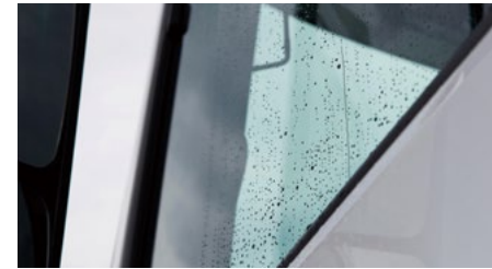
Water-repellent Coated Pull-down Door Glasses
