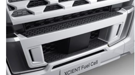
FIXED STEP BUMPER Steps provide secure footholds for easy windshield access.
