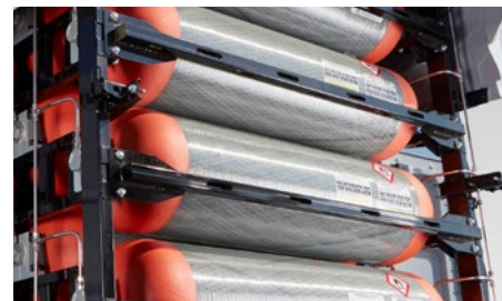
HYDROGEN TANK 1 68.6 kg H 2 (700 bar)
