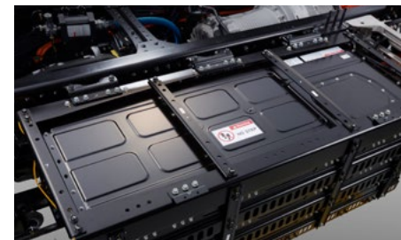
BATTERY 3 72 kWh (3 x 24 kWh each)
