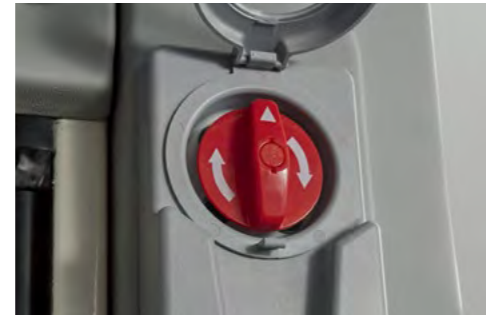
Middle Door Manual Opening / Closing Device
