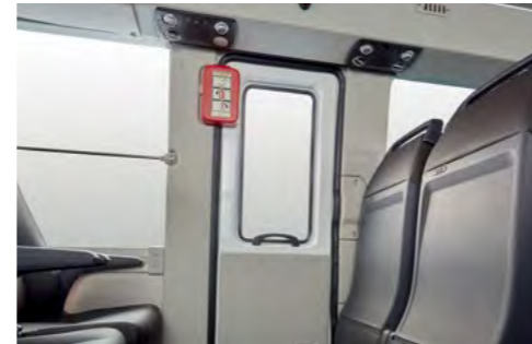
Emergency Exit Door
