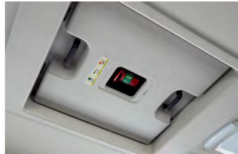
Emergency Escape Hatch and Flashlight
