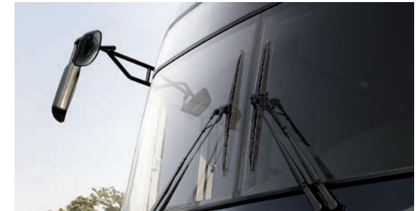
Front Two-Piece Glasses, Parallel Wipers, and Mirrors with LED Turn Signal Lamps
